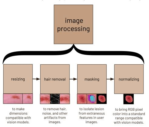
Note: Our application applies this image processing to user image before feeding it into the classification model. Hair removal and masking ensure stability across diverse user images.
